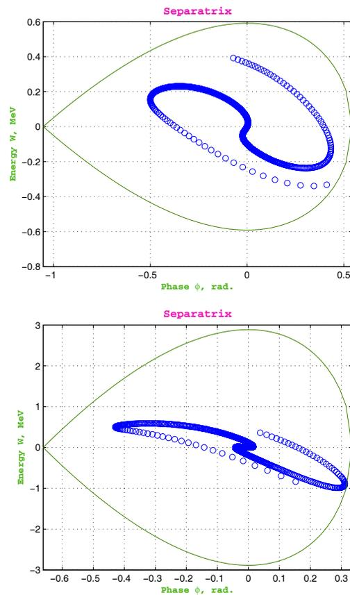
Figure 3: Separatrix and energy-phase distribution of the particle beam at the output of buncher (upper plot) and output of structure (lower plot)
