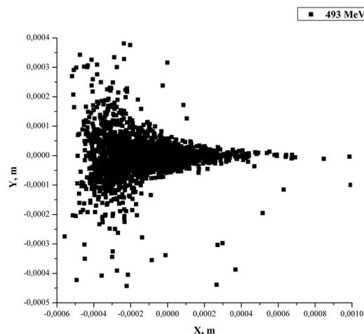
Figure 9: Beam cross-section on exit the D channel.
