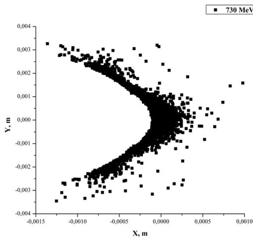
Figure 3: Beam cross-section on exit the B channel.
