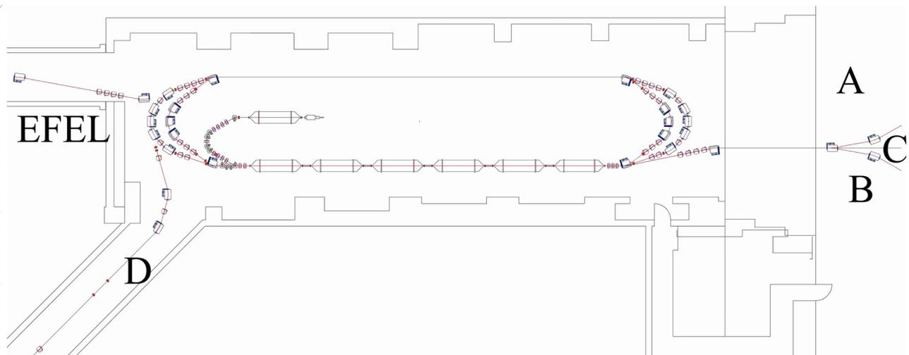
Figure 1: Beam output channels on SALO recirculator.
