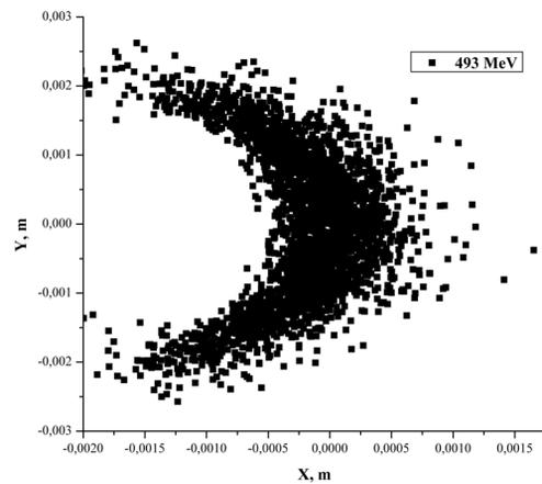
Figure 6: Beam cross-section on an input in the FEEL channel.
