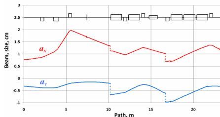
Figure 7: The beam envelopes along the channel.
