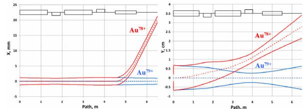
Figure 9: The separation of  $Au^{78+}$  ion beam.
