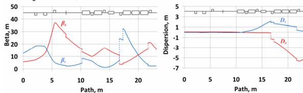
Figure 6: The optical functions of the beam.
