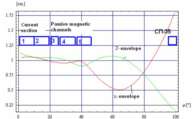
Fig 6:  $2\sigma$  beam rms-envelopes inside the extraction system
