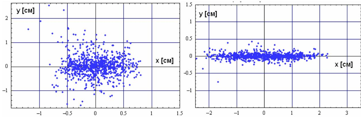
Fig 7: Beam profiles (calculated) at point A (see Figure 1) and at the entrance to the SP-35 magnet
