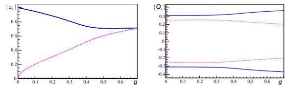
Figure 3: Dependences of  $|z_k|$  and  $\{Q_k\}$  on gain  $g$ . There are four
