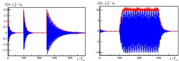
Figure 2: Beam response signal (solid blue lines) and its envelope (dashed red lines) on two  $\delta$ -kicks (left), harmonic impulse (right) and damped injection oscillations at  $t = 0$
