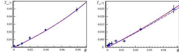
Figure 5: Calculated decrements (curves) and results of measurements for vertical (left) and horizontal (right) feedback chains of the LHC Damper at the energy of 3.5 TeV
