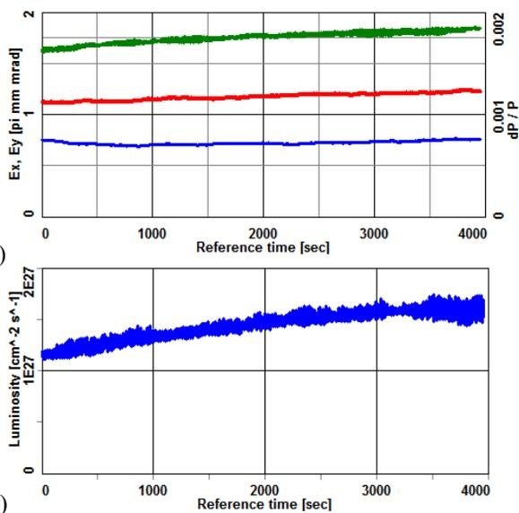
Figure 5: Evolution of beam parameters for ion energy 4.5 GeV/u and electron current 0.33 A: a) green line – momentum spread, blue and red – horizontal and vertical emittances, b) luminosity.
