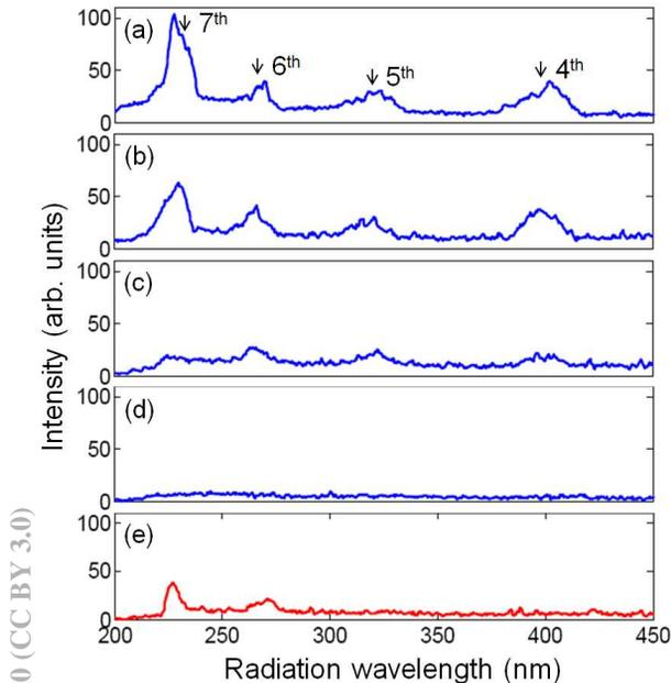
Figure 1: Spectrum of the radiation for various TCAV1 voltage: (a)  $V=0$ ; (b)  $V=85 \text{ kV}$ ; (c)  $V=170 \text{ kV}$ ; (d)  $V=255 \text{ kV}$ . The beam slice energy spread increases as we increase TCAV1 voltage. (a)-(d) are the HGHG signals when only the 1590 nm laser is on and (e) is EEHG signal at  $V=255 \text{ kV}$  with both lasers on.
