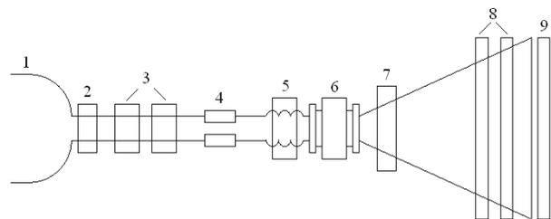
Figure 1: 1 – accelerating structure, 2 – control magnet, 3 – quadrupole doublet, 4 – diaphragm, 5 – bellows unit with correction system of scanning field, 6 – scanning chamber with scanning electromagnet, 7 – transverse beam scanning system, 8 – Panovsky lenses, 9 – converter.
