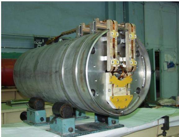
Figure 1: SIS300 SC high field fast cycling dipole model.
