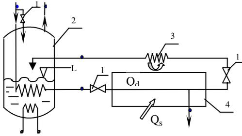
Figure 7: Flow scheme proposed for cryostating the string of SIS300 superconducting magnets. 1 - valves, 2 - subcooler, 3 - heat exchanger, 4 - SC magnets string.
