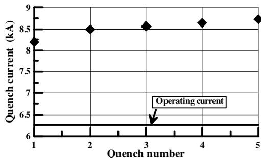
Figure 5: Quadrupole quench current vs. quench number.
