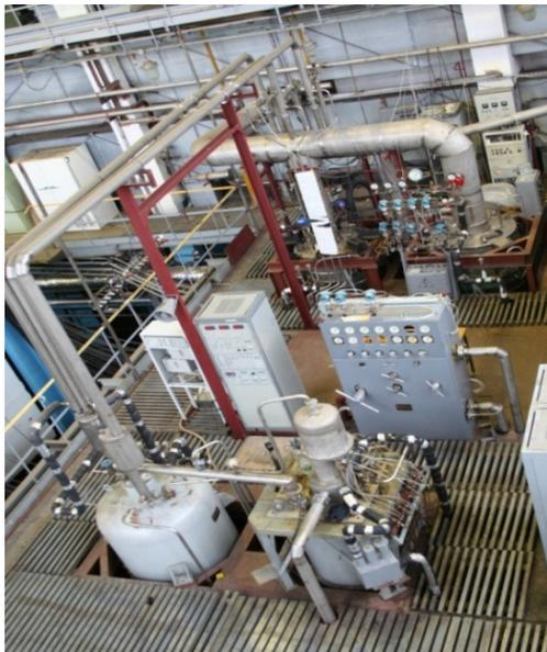
Figure 8: Cryogenic plant and large helium heat exchanger of superfluid refrigerator system of kaon channel.
