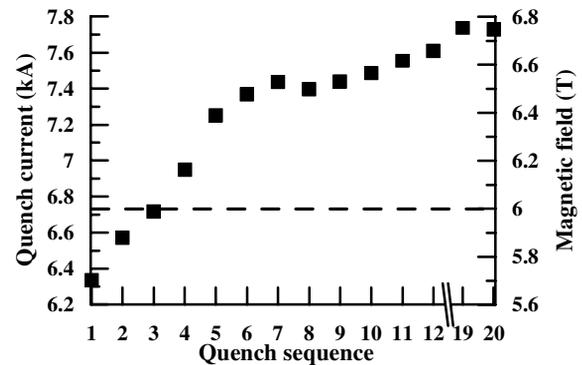
Figure 2: Training curve of the SIS300 dipole model.
