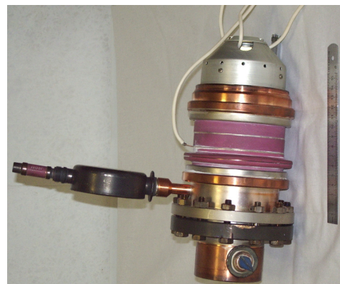
Figure 2: Electron gun after manufacturing.
