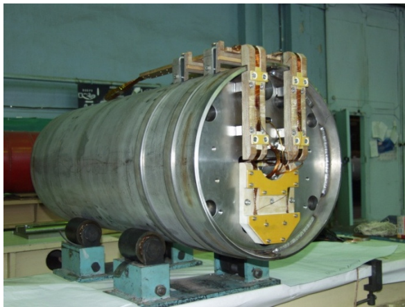
Figure 1: SIS300 SC high field fast cycling dipole model.
