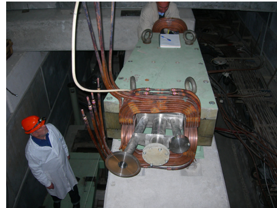
Figure 2: 4MC magnet assembly view downstream.
