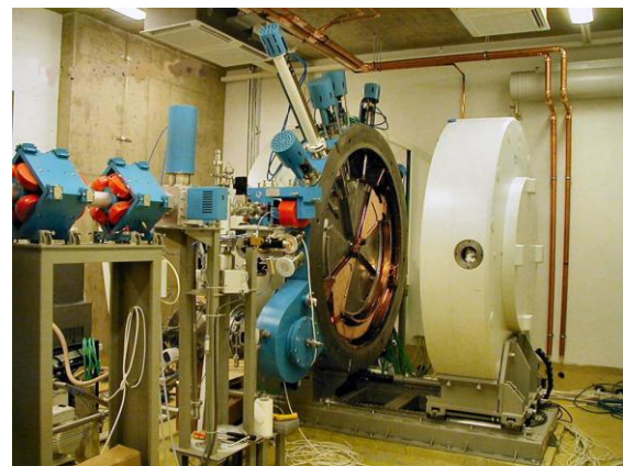
Figure 1: The CC-18/9 cyclotron installed in Turku (Finland).
