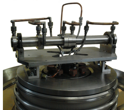
Fig. 2. New Ø16-mm stripping target placed on the feedthrough insulator.
