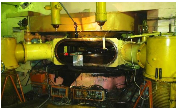
Figure 1: Cyclotron U-150 during the measurements of the magnetic field.
