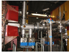
Figure 14: Energy-degrader inner target IT#28 (beryllium, thickness 4.0 mm, height 10 mm) for carbon beam and the IT outer assembly at SS#28.
