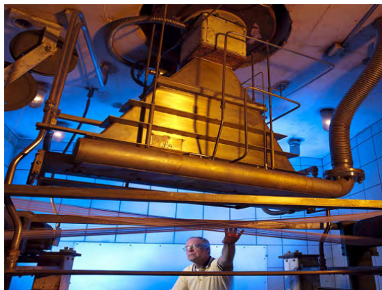
Figure 11: Electron beam cross-linking of polymers improves heat resistance of coatings for wires and cables.
