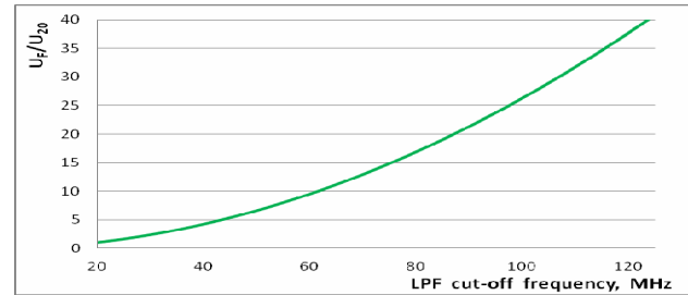
Fig.1. Calculated dependence of the relative signal amplitude in the LPF output U_F / U_0 on the F_{LPF} .
