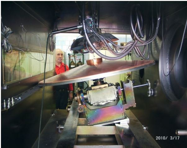
Figure 2: The left side wall with the cone nose installed into the vacuum chamber before the electron beam welding.
