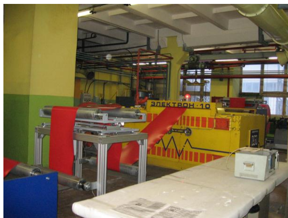
Figure 7: The «Electron-10» accelerator at the plastic materials production plant, Izhevsk.
