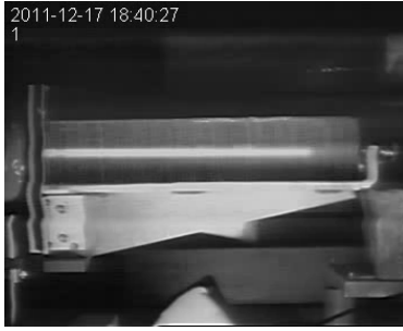
Figure 7: Finite range (30 cm ca) of extracted carbon beam through a plastic scintillator at 455 MeV/u.
