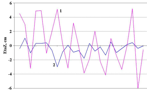
Figure 1: Vertical dispersion function at SIBERIA-2 BPMs before correction (1) and after it (2).
