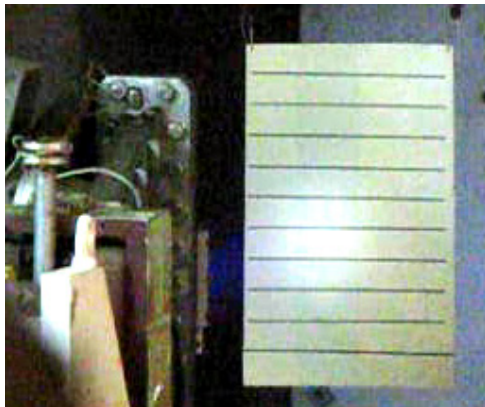
Figure 7: Electron beam image on plastic (distance between lines – 50 mm).
