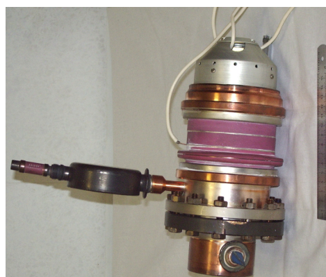
Figure 2: Electron gun after manufacturing.
