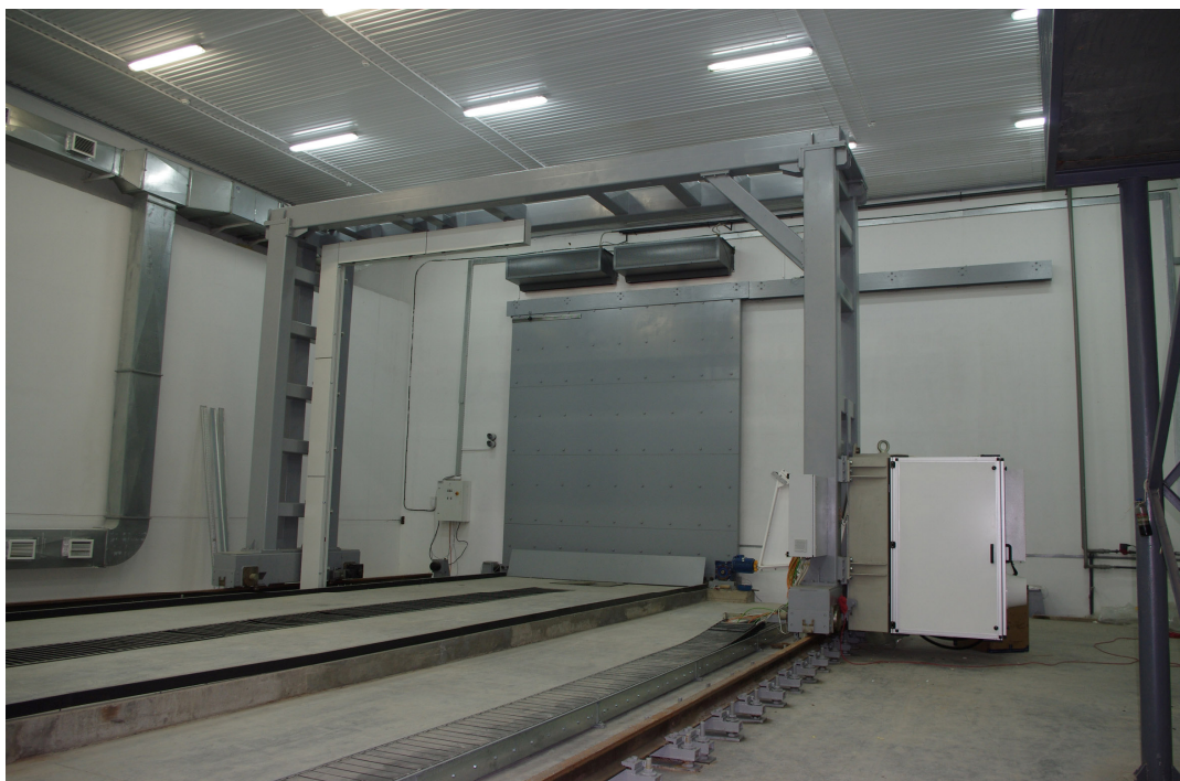
Figure 1: The IDK-6/9MeV accelerator in a customs inspection system.
