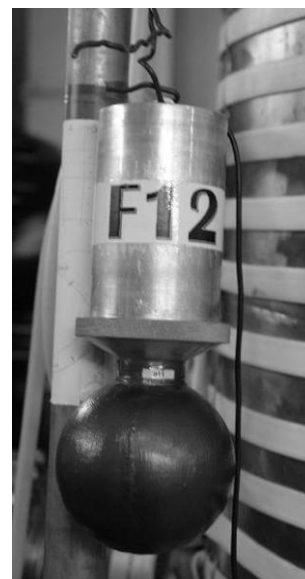
Fig.2. Detection unit dose power of photon radiation.
