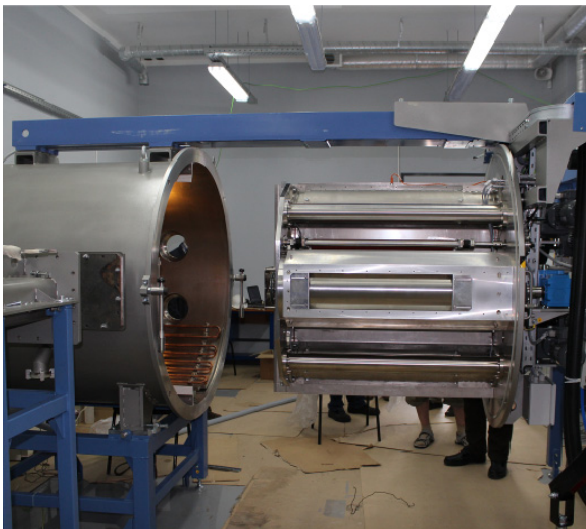
Figure 4: The facility for irradiation of polymer films at the DC-110 cyclotron
