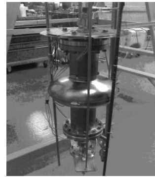
Figure 5: Vertical stand for 1-cell testing.
