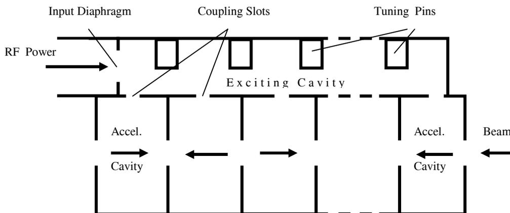
Figure.1: Conceptual scheme of the PCAS
