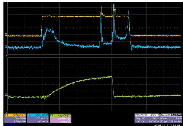
Figure 3c: Regime with breakdowns in several accelerating cavities. F1 – RF power from klystron, 1.6 MW, pulse duration 5  $\mu$ s; F3 – reflected signal; F4 – stored RF energy in 5-th accelerating cavity.
