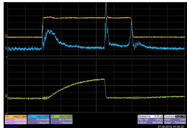
Figure 3b: Breakdown in the 5-th accelerating cavity.
