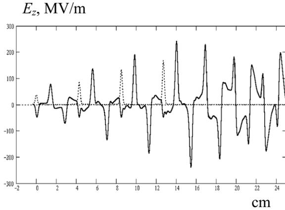
Figure 2: Longitudinal field structure behind four bunch train.
