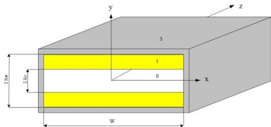
Figure 1: A rectangular dielectric based accelerating structure.
