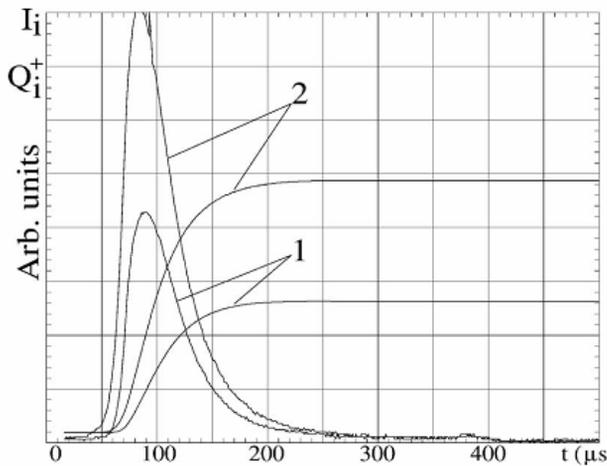
Figure 4:  $\text{Kr}^{27+}$  ion pulses: 1 – cooling “off”; 2 – cooling “on.”
