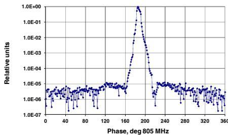
Figure 6: Longitudinal profile combined from several measurements with gains ranging within 3500.
