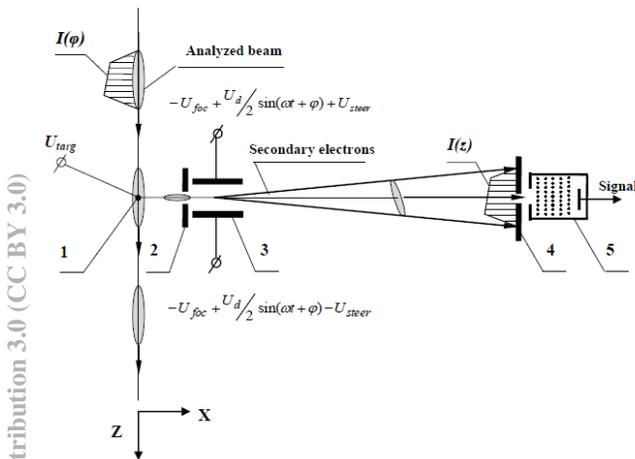
Figure 1: Principle of operation of Bunch Shape Monitor (1 - target, 2 - input collimator, 3 - rf deflector combined with electrostatic lens, 4 - output collimator, 5 - electron collector).
