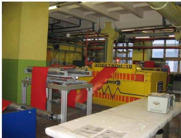
Figure 7: The «Electron-10» accelerator at the plastic materials production plant, Izhevsk.
