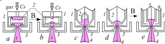
Figure 1:: Schematic diagrams of the basic versions of CSPS.: a) plain magnetron (planotron); b) magnetrons with geometrical focusing; c) Penning discharge SPS (Dudnikov type source) was adopted for injection into ISIS; d) semiplanotron; e) hollow cathode SPS
