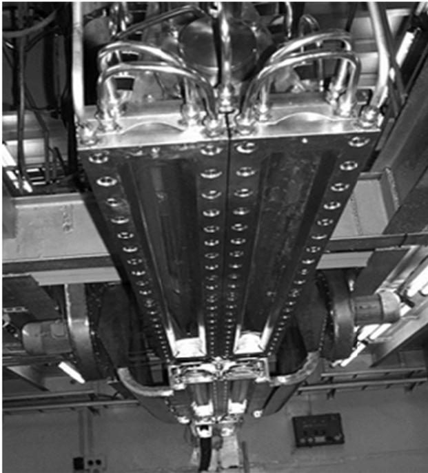
Figure 2. Double window extraction device of ELV-12 accelerator.
