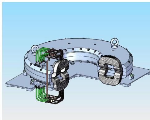
Figure 4: The analyzing magnet.
