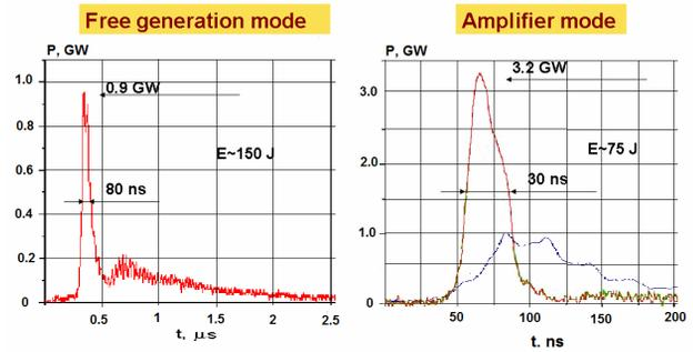
Figure 9: Pulses of L100 radiation for auto-generator and amplifier modes of laser operation.
