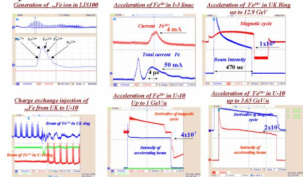
Figure 6: Fe-nuclei acceleration up to relativistic energy.
