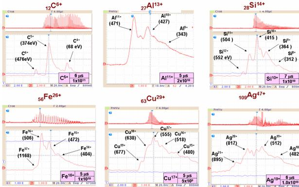
Figure 4: Ions generation in LIS with laser L100.
