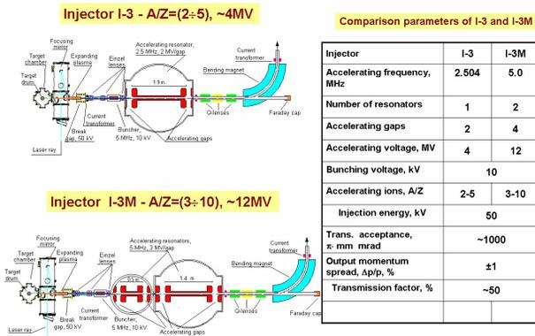
Figure 11: Scheme of ion injector I-3 upgrading.
