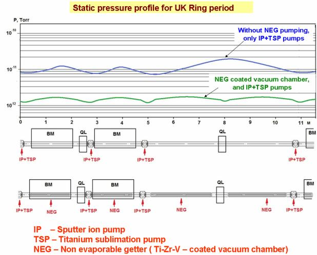
Figure 12: Scheme of UK Ring vacuum pumping.
