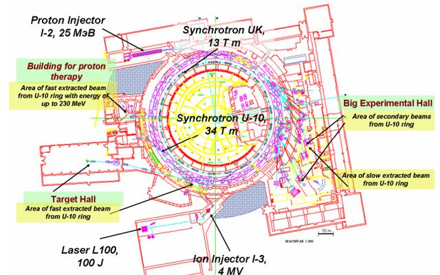
Figure 1: Layout of ITEP-TWAC Facility.
