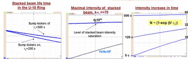
Figure 7: Optimization of carbon nuclei stacking in U-10 Ring by scheme of C<sup>4+</sup> => C<sup>6+</sup>.
