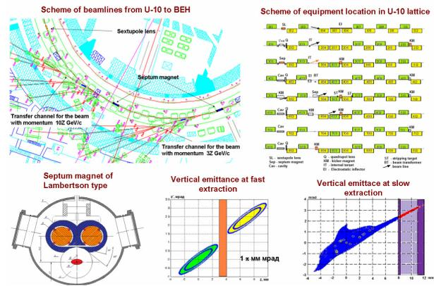
Figure 13: Combined extraction of beam from U-10 Ring.
