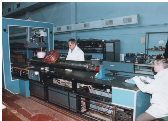
Figure 2: Machine for 6 m length SC coil winding.
