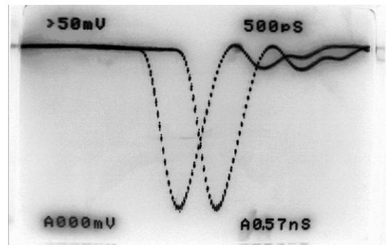
Figure 5: Oscillogram of a current pulse in the collector circuit (the same pulse is depicted with a 0,57 ns shift in order to define the time-response characteristic).
