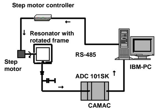
Figure 2: A scheme of the mechanism for resonator autotuning.
