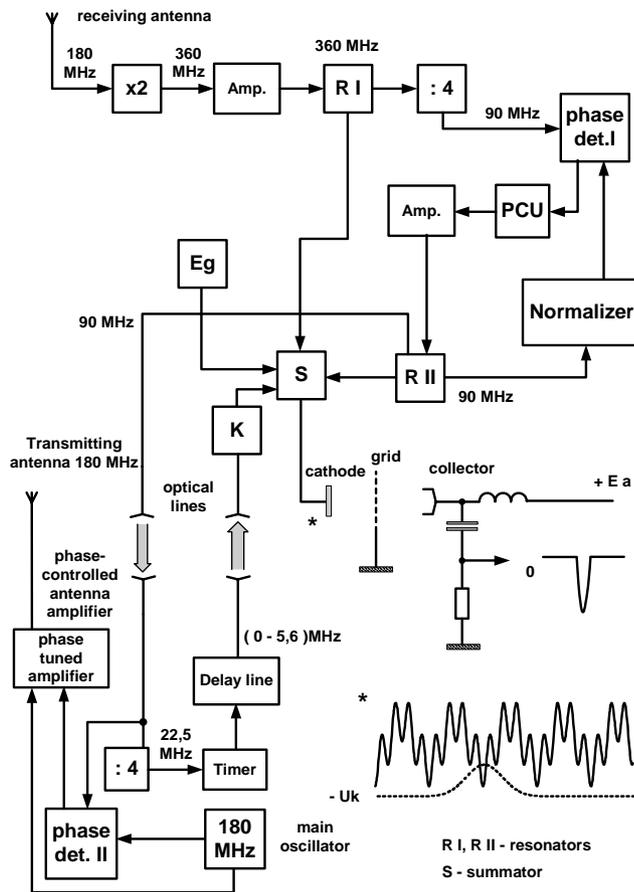
Figure 3: Scheme of links of main elements of the electron source.
