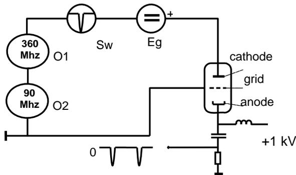
Figure 1: Basic diagram of current pulse generation.
