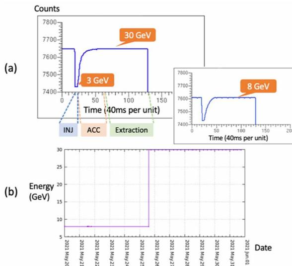
Figure 6: (a) The frequency shift of the LLRF signal is observed by the read-back system. In every machine cycle, 3-GeV protons are injected into MR, then accelerated up to 30-GeV or 8-GeV. (b) 10-day history of the MR energy, which is deduced from the observed LLRF patterns. The energy was changed from 8-GeV to 30-GeV on May 25, 2022.
