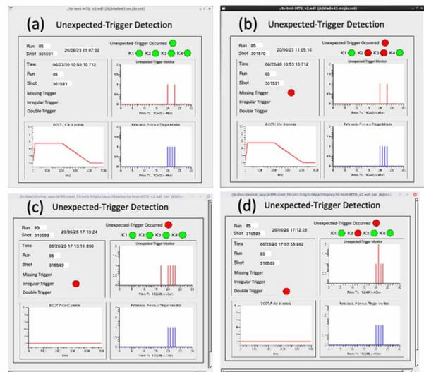
Figure 2: Test results of the prototype system using a dummy injection-kicker signal. Red means an observed signal, blue means a reference signal. Screenshots for (a) normal event with the saved information of the last fault event, (b) a missing-trigger event, (c) an irregular-trigger event, and (d) a double-trigger event.
