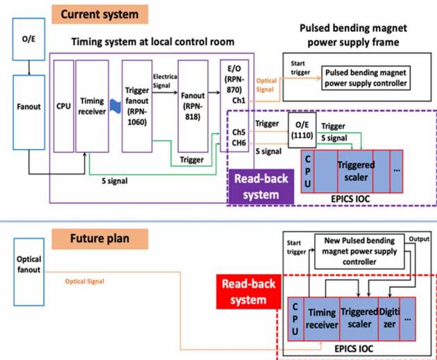
Figure 8: Comparison of current and future timing read-back systems for pulsed bending magnet trigger.
