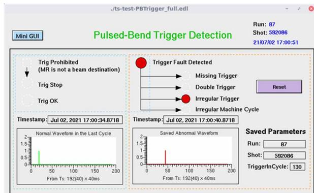
Figure 4: The GUI screenshot of pulsed bending magnet trigger with a simulated irregular-trigger event.
