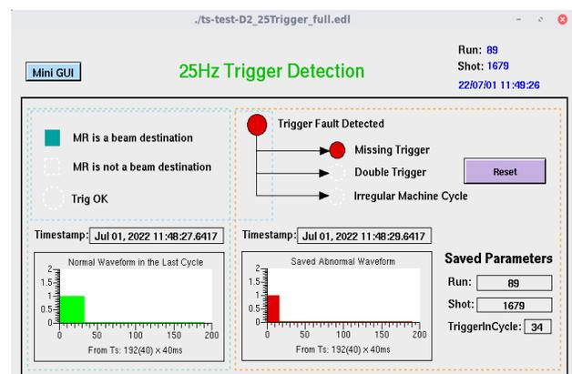
Figure 3: The GUI screenshot of 25-Hz trigger clock for one of power-supply buildings. The indicated error is caused by a simulated missing-trigger signal. Red means an observed signal, green means a reference signal.
