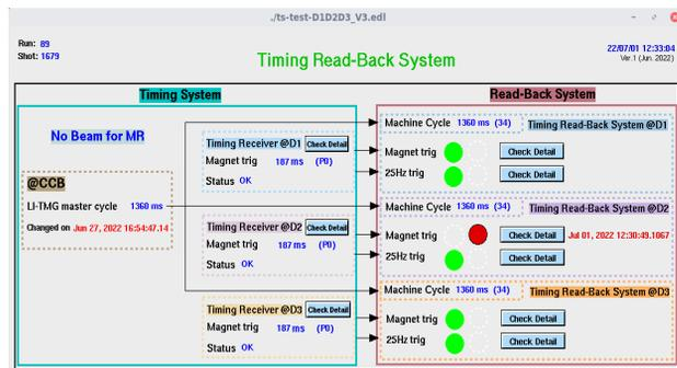
Figure 5: The GUI screenshot of 25-Hz trigger clock and magnet power-supply trigger. The “Timing System” part shows timing system related information. The “Read-Back System” part shows the observed signal status of three power-supply buildings. The indicated error is caused by a simulated missing-trigger signal.
