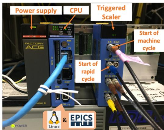
Figure 1: Hardware setup of the prototype system.
