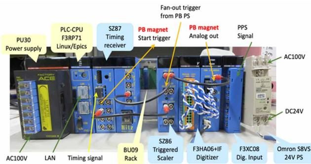
Figure 7: The picture of the read-back system with a new PLC-type timing receiver.
