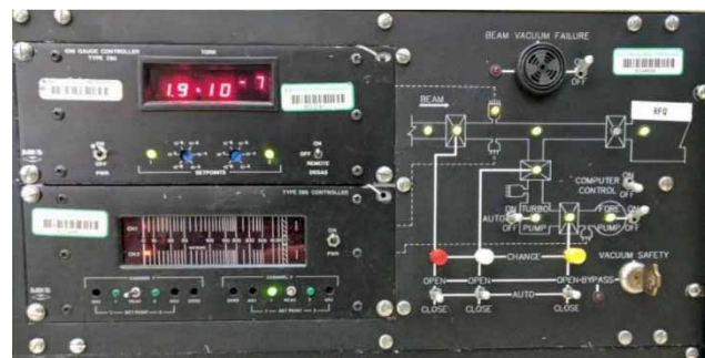
Figure 1: Hardware-based vacuum Control Chassis with adjustable vacuum set point switches.
