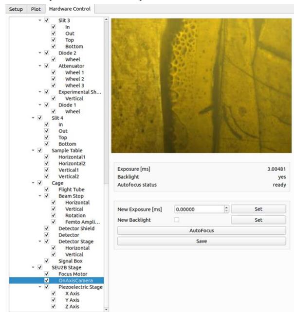
Figure 3: BECQUEREL GUI (SEU2B camera control tab).
