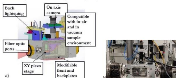
Figure 2: Sample Exposure Unit a) Model, b) Installation at the Beamline.
