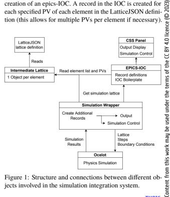
Figure 1: Structure and connections between different ob jects involved in the simulation integration system.
