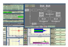
Figure 1: Native LLRF GUI. Visible is the top level control, the network analyser and the waveform acquisition tools.
