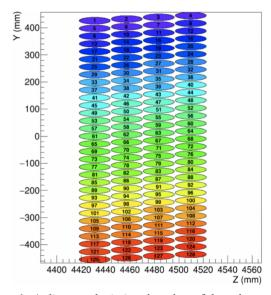
Figure 1: A diagram depicting the tubes of the subset of the LoKI detector tested at ISIS in March 2022.
