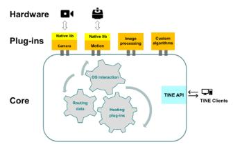
Figure 1: Architecture of the Smart Video System.
