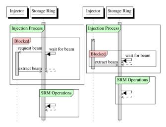
Figure 1: Sequence diagram of a strong coupling (left) and weak coupling (right).
