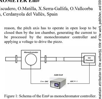
Figure 1: Schema of the Em# as monochromator controller.
