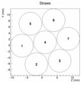
Figure 2: A diagram depicting the straws within each tube of the LoKI detector.
