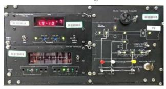
Figure 1: Hardware-based vacuum Control Chassis with adjustable vacuum set point switches.
