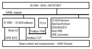
Figure 1: Current GANIL control system architecture.
