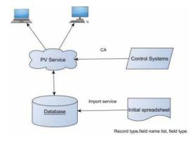
Figure 2: System Architecture.
