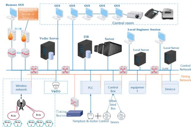
Figure 1: Control system hardware scope of view.
