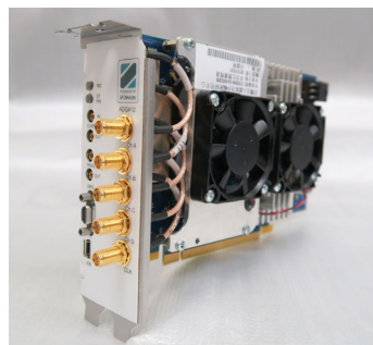
Figure 6: Outward of ADQ412 with PCIe form factor.
