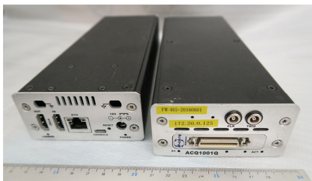
Figure 4: Outward of ACQ1001 with FMC module.
