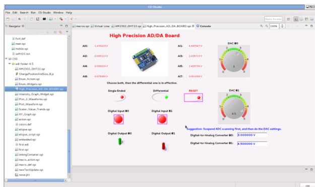
Figure 4: Graphic user interface of AD/DA board in the control console.
