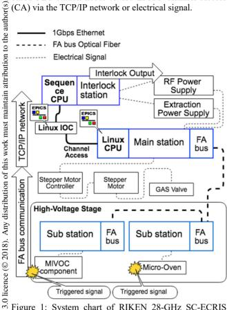
Figure 1: System chart of RIKEN 28-GHz SC-ECRIS control system. CA protocol is utilized for operation services and triggered signal.
