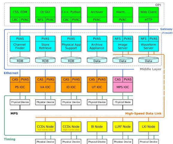
Figure 1: Architecture of the control system.
