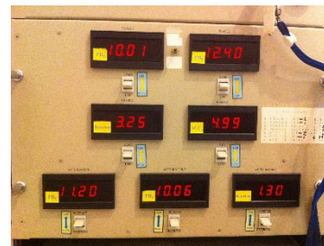
Figure 2: Electronic front panel display of the phase shifters and amplitude attenuators as DC voltages.
