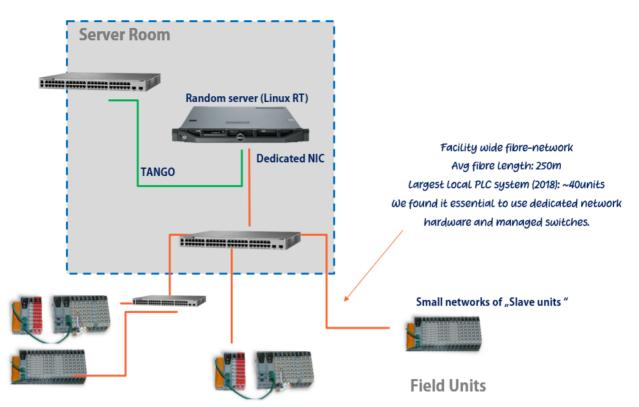
Figure 2: Alternative concept for propagating Industrial Ethernet systems.
