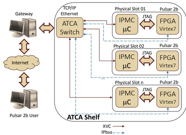
Figure 3: Connections between developer and FPGA using the XVC service and IPbus.
