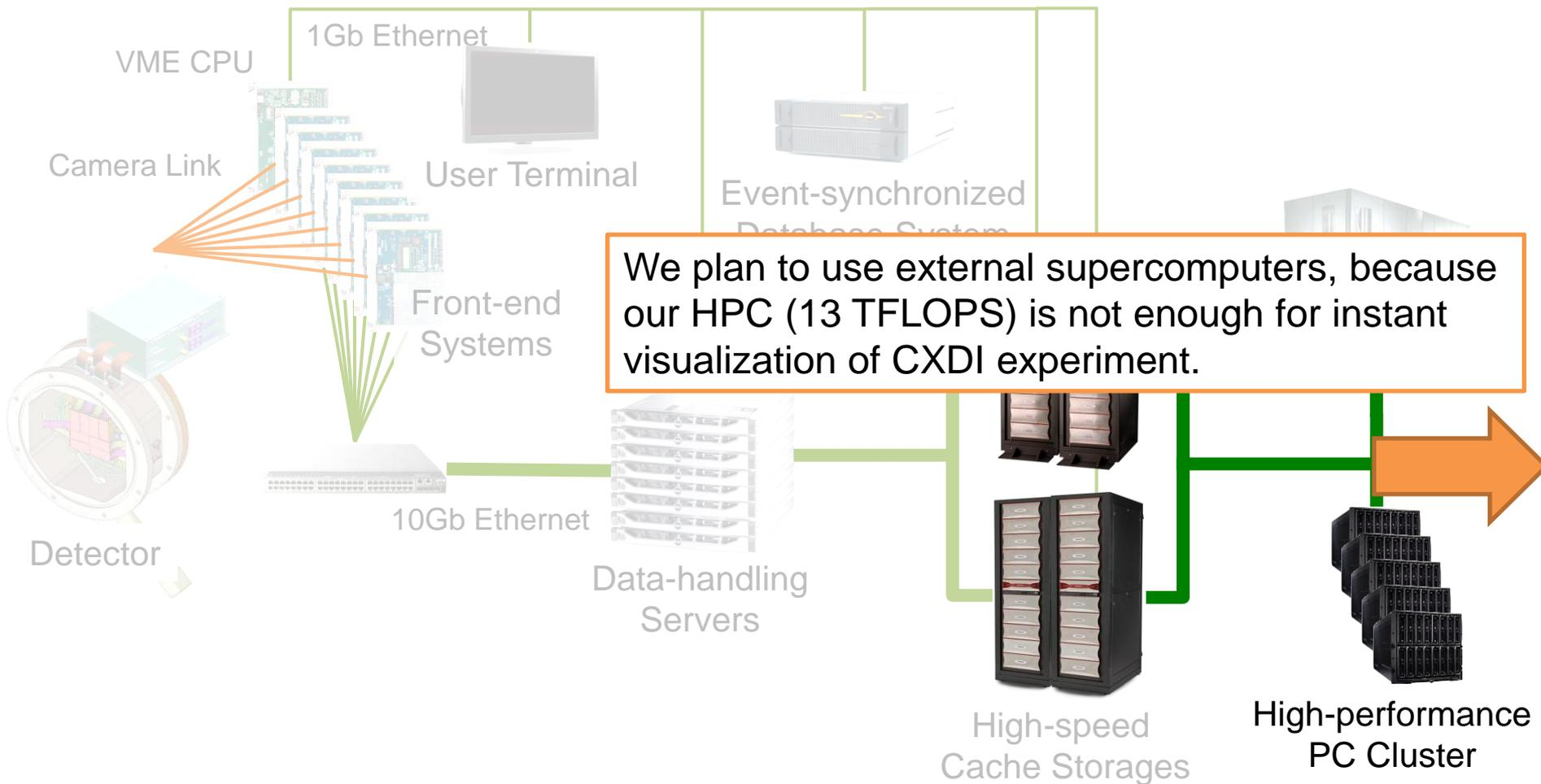
We plan to use external supercomputers, because our HPC (13 TFLOPS) is not enough for instant visualization of CXDI experiment.
