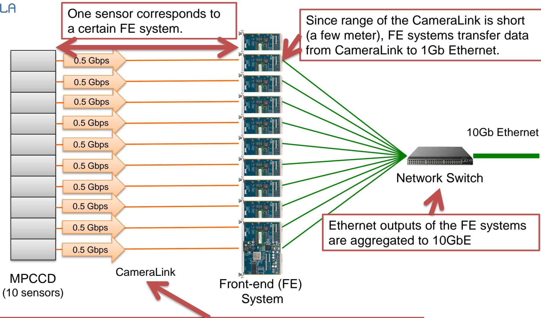
We choose CameraLink as digital interface between MPCCD and FE system. Because we can use other commercial cameras.
