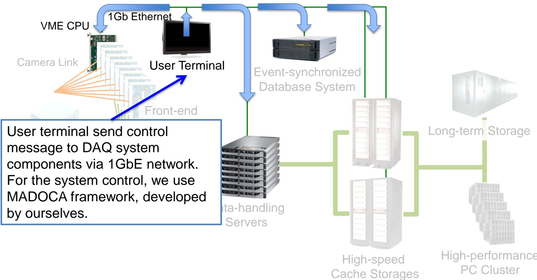
User terminal send control message to DAQ system components via 1GbE network. For the system control, we use MADOCA framework, developed by ourselves.
