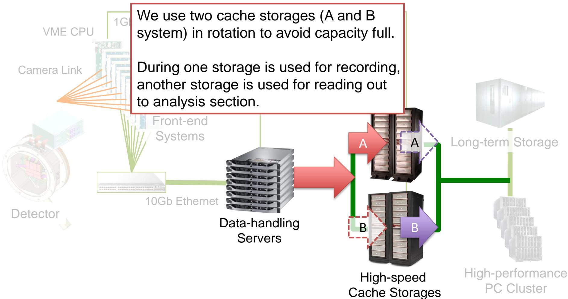
We use two cache storages (A and B system) in rotation to avoid capacity full.
