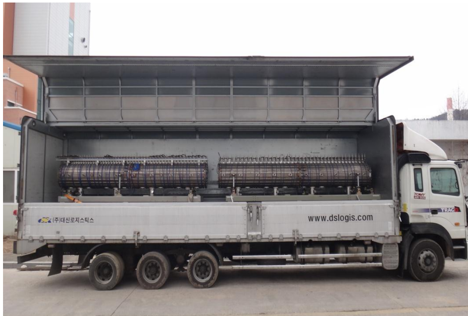
DTL tanks inside vibration free truck
