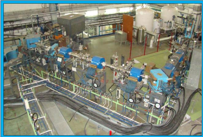
Figure 1: ECR Ion Source and Horizontal Injection Line
