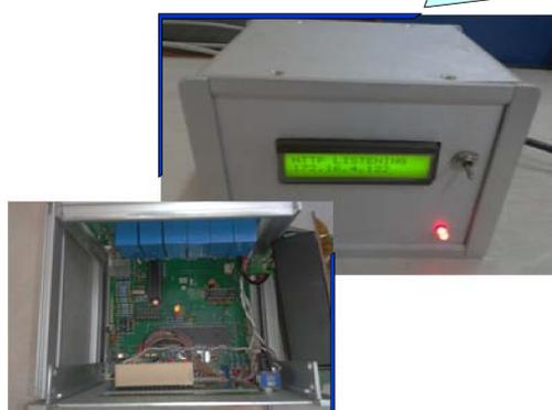
Figure 3: Assembled Ethernet Module
