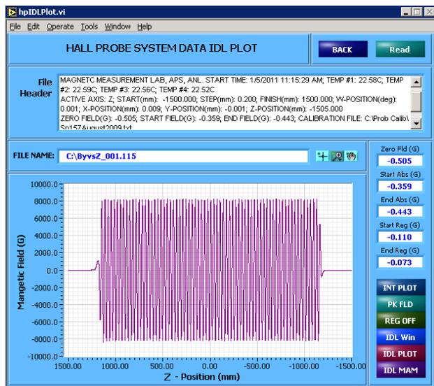
Figure 3: APS ID magnetic field measurements.
