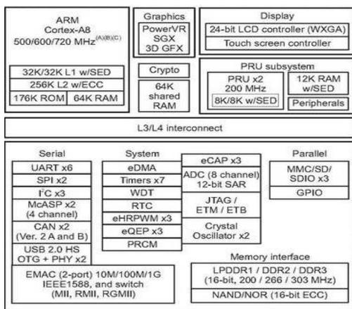
Figure 2: AM335x SOC architecture.
