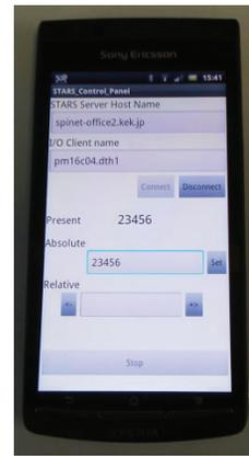
Figure 5: Motor Control Panel on a smart phone.
