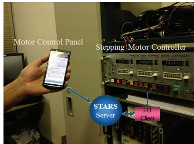
Figure 6: Stepping motor controller operated by the Motor Control Panel through STARS.
