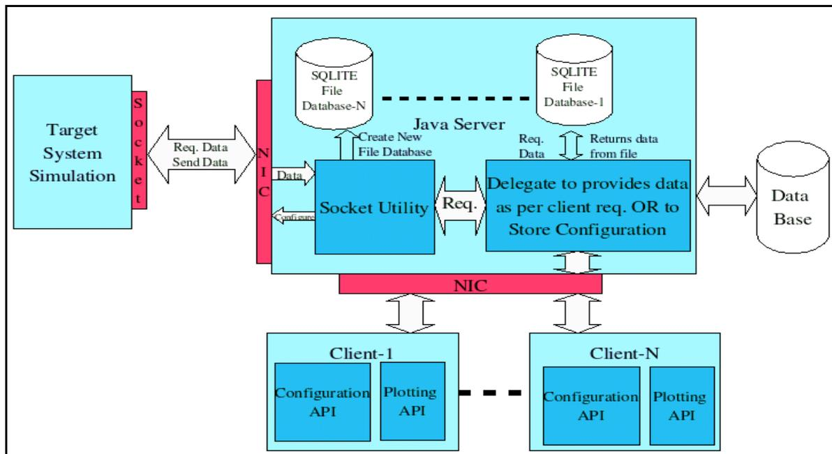
Figure 2: Application architecture of the data acquisition software system.
