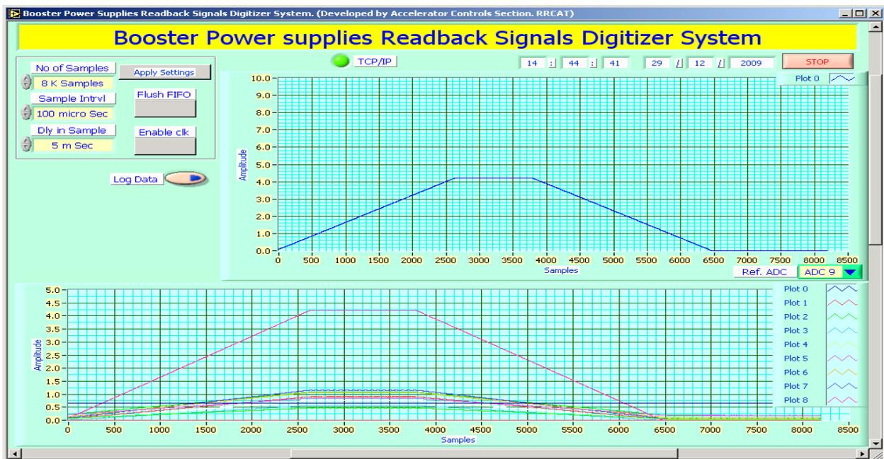
Figure 2: Graphical representation of captured ramp data waveforms.
