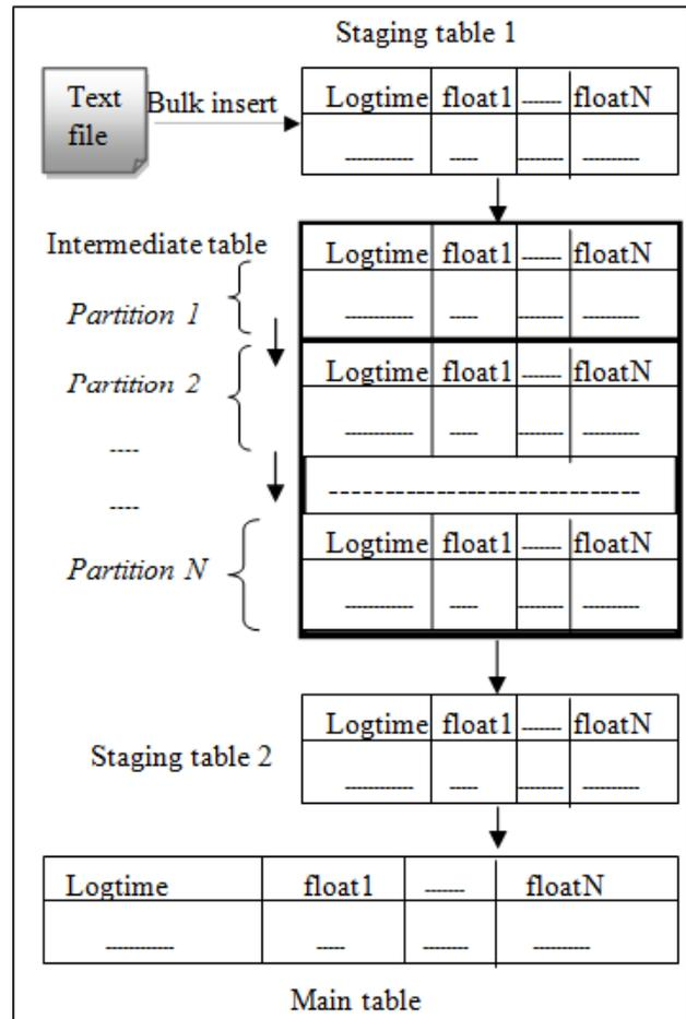
Figure 2: Data flow cycle for analog parameters.
