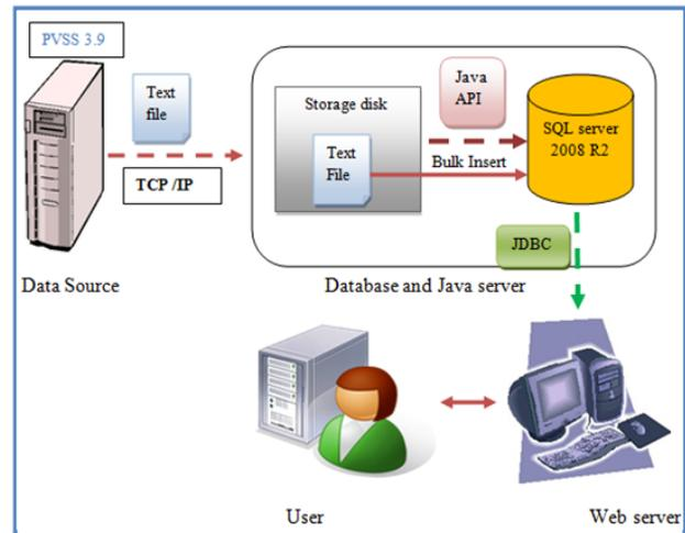
Figure 1: High level layout of data logging architecture.
