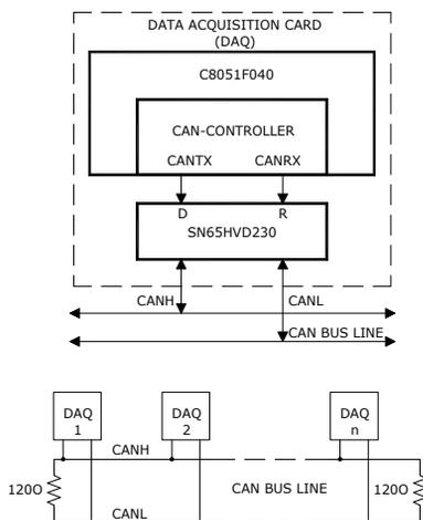
Figure 2: Details of typical CAN DAQ node.
