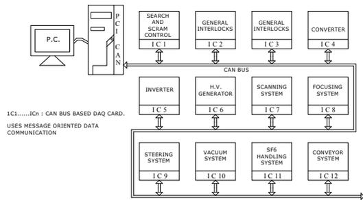
Figure 3: Schematic of the control system.
