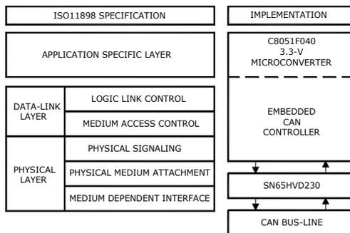
Figure 1 : The Layered ISO 11898 Standard Architecture.
