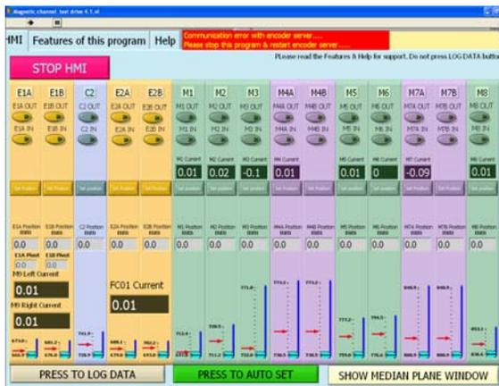
Figure 7: HMI for the drive control system.
