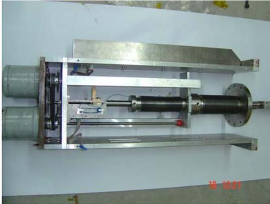
Figure 4: Motor drive for magnetic channel M4.
