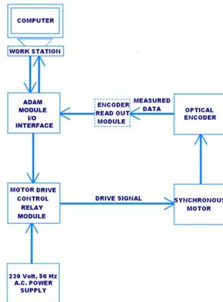
Figure 5: Block diagram of drive system.
