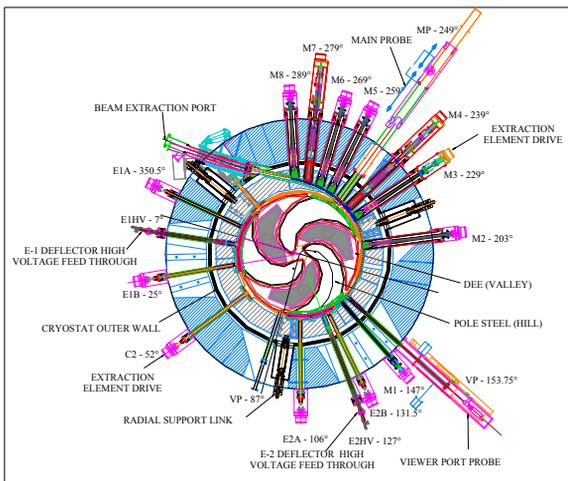
Figure 1: Extraction system layout.
