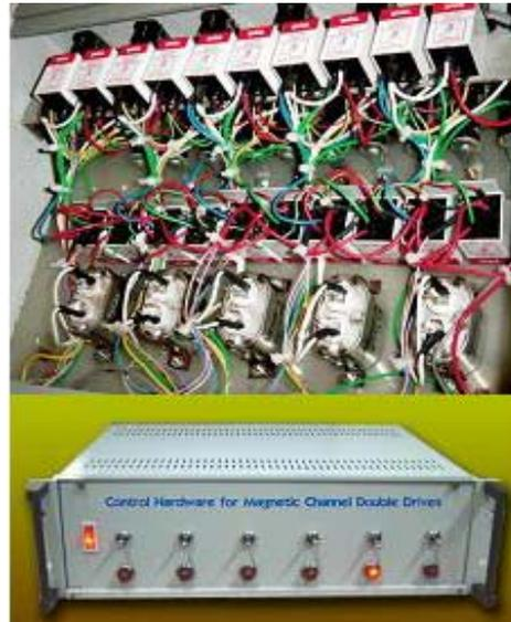
Figure 6: Internal & external view of the control module.
