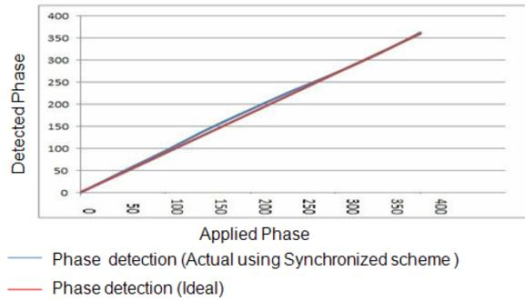
Figure 3: Phase detection characterization.
