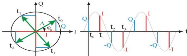
Figure 2: I/Q detection scheme.
