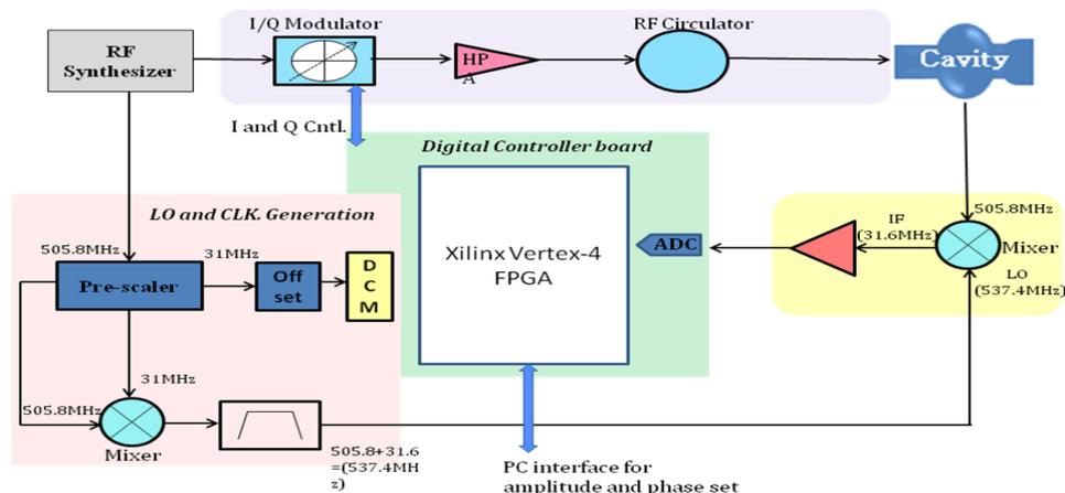
Figure 1: Block Diagram of Digital Feed Back Control System.
