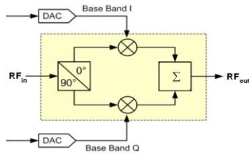
Figure 6: Typical Block diagram of I/Q modulator.
