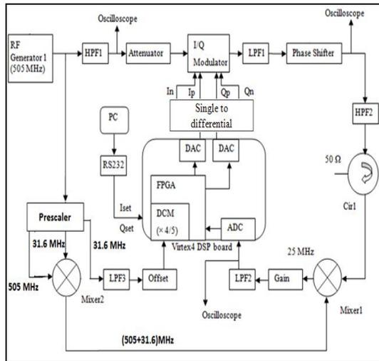
Figure 7: Block diagram of the test setup.
