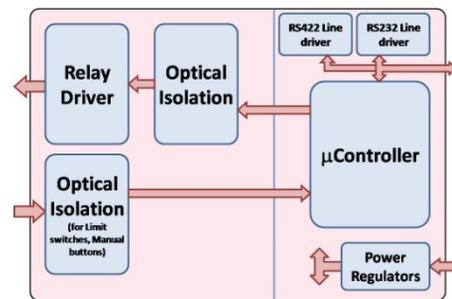
Figure 6: Circuit diagram of Input-Output module.
