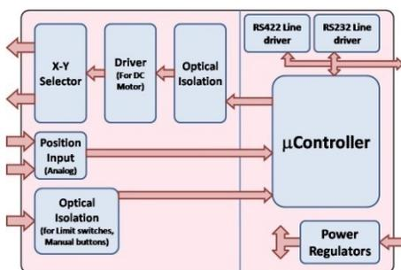
Figure 4: Block diagram of X-Y Slit module.
