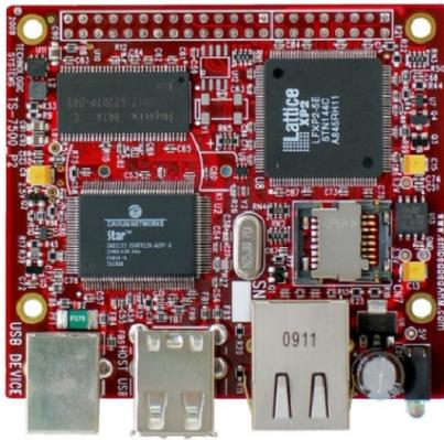
Figure 2: ARM-9 based Single Board Computer.
