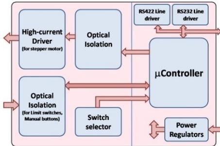
Figure 3: Block diagram of Stepper Motor module.
