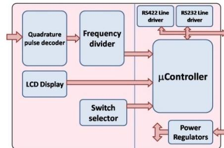
Figure 5: Block diagram of Encoder Read-out module.
