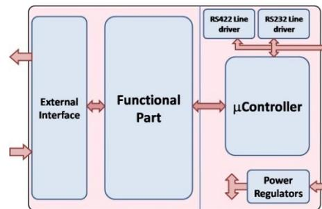
Figure 1: Block diagram of the basic scheme of module.
