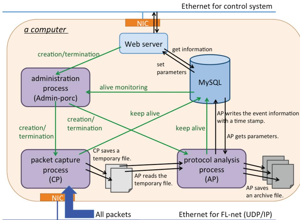
Figure 3: Schematic view of the monitoring system for the FL-net protocol.
