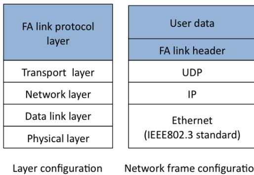
Figure 2: The layer configuration and network frame configuration of the FL-net protocol.
