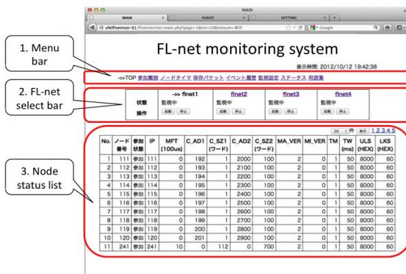
Figure 4: The main page of the Web browser. The language is set to Japanese. The red line around the box No. 1 area indicates the menu bar used for browsing. The No. 2 area is the FL-net select bar, which can start/stop the monitoring by the click of a button. Finally, the No. 3 area shows the node status and configuration list.
