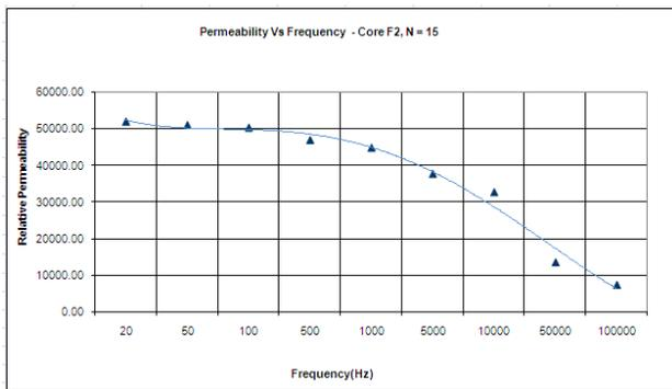
Figure 2: Permeability vs. frequency curve.
