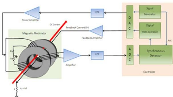
Figure 6: Magnetic modulator in a closed loop – low frequency channel of DCCT.
