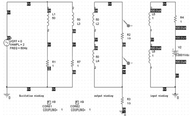
Figure 3: Magnetic modulator circuit.
